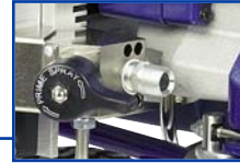
Optimized fluid passages 1/2" porting Smooth fluid passages 1/2" hose coupled with a 3,3 meter whip hose for flexibility
