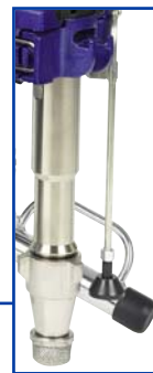
HD Endurance™ pump Chromex rod Outlasts standard chromed pistons Lowered inlet check Brings the suction power down where it is needed Ceramic balls Higher resistance against wear with abrasive materials Spring loaded Fast priming and fast closing of the inlet ball for improved performance Extra large fluid passages To handle thicker products
