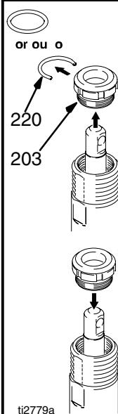
Remove throat nut spacer (220) when pump packings begin to leak after much use. Then tighten packing nut down until leakage stops or lessens. This allows approximately 100 gallons of additional operation before a repacking is required.
