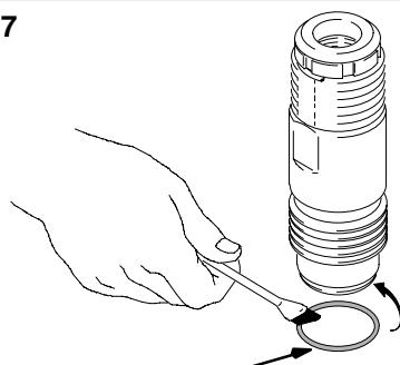
Grease and place on O.D. ring groove
