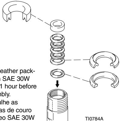
Soak leather packings in SAE 30W oil for 1 hour before assembly.
