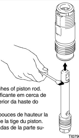
Grease top two inches of piston rod.
