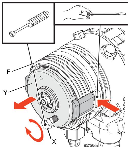
**NOTE:** If excessive force is required to remove the PC fluid cartridge, use the provided nut driver and jack screw (X) to lift the cartridge out of the fluid housing (F).
