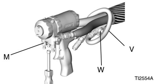
5. Connect the air line quick coupler (D). Turn on air. Open air valve (W). Air should flow from the mix chamber nozzle (N).
