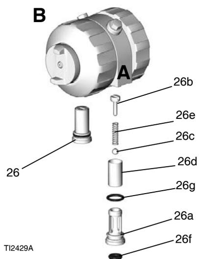
7. Reassemble check valves. Screw (26b) should be flush (within 1/16 in. or 1.5 mm) of housing (26a) surface. Liberally lubricate o-rings (26f, 26g) and carefully reinstall in fluid housing.
