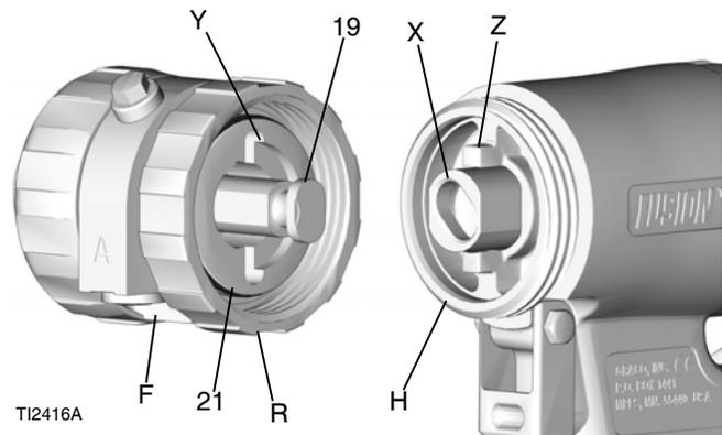
5. Turn fluid housing 1/8 turn clockwise to engage slots (Y) and tabs (Z). Push on front end to ensure it is properly seated. Continue screwing lock ring (R) onto handle (H) very securely. When properly assembled, lock ring is snug against handle.
