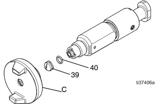
**NOTE:** If tip is stuck, pry off with small screwdriver or pull off with pliers. Tip is hardened to resist damage.
