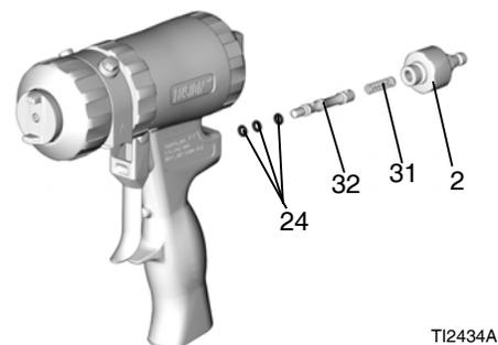
4. Liberally lubricate o-rings and reassemble. Torque plug (2) to 125-135 in-lb (14-15 N•m).
