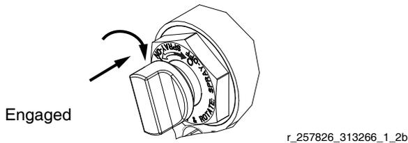
**To disengage the piston safety lock:** Push knob in and turn counterclockwise until it pops out. There will be a gap between knob and gun body.
