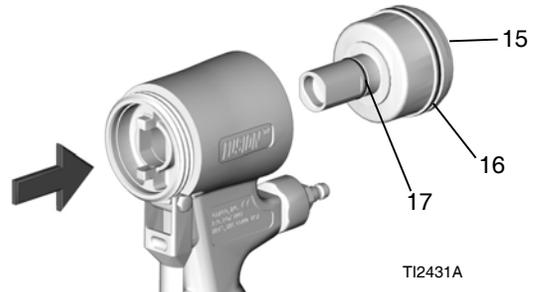
7. Liberally lubricate piston o-rings. Reinstall piston. Shaft is keyed for proper assembly. Push firmly to seat piston.
