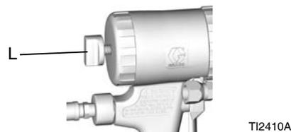
4. Trigger the gun onto cardboard or into a waste container to relieve pressure.
